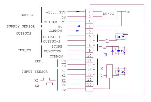
It is possible to connect an encoder with a 5V output as well as a 24V output.
